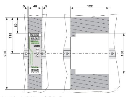
Slim-style installation: Installation depth 125 mm (+ DIN rail) (state at delivery)
