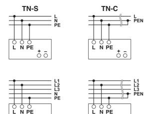
The 100 ... 240 V AC connection is established using the L, N and PE screw connections.
