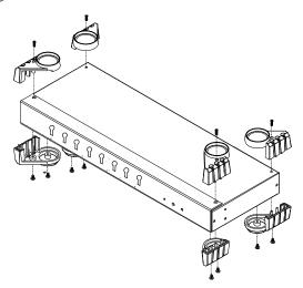
2. Screw the mounting brackets into the sides of the unit, as shown in the diagram below:
