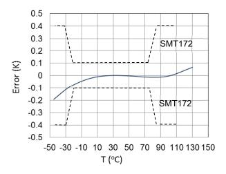
Inaccuracy vs. temperature (TO18)
