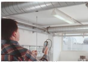
testo 425, e.g. for setting the air input in a kitchen
