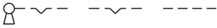
19 Keylock switch actuator 3 positions page 16 | Keylock switch actuator 3 positions, flush mounting page 22
