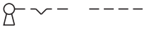
17 Keylock switch actuator 2 positions page 15 | Keylock switch actuator 2 positions, flush mounting page 21
