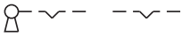
18 Keylock switch actuator 3 positions page 16 | Keylock switch actuator 3 positions, flush mounting page 22
