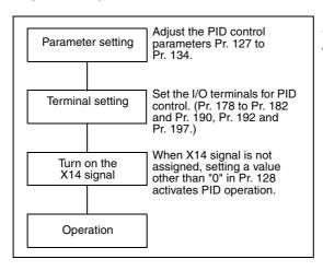
Fig. 6-128: Adjustment procedure
