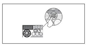
Fig. 7-1: Resetting the inverter by using the operation panel
