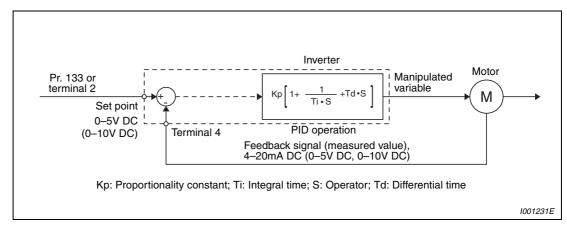
Fig. 6-119: System configuration when Pr. 128 = 20 or 21 (set/feedback value at the inverter)
