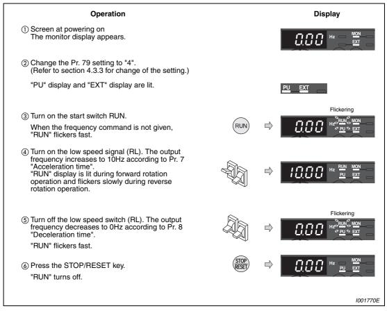
Fig. 5-15: Operate the inverter by using multi-speed setting
