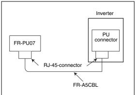
Fig. 6-97: Connecting the PU to the PU connector
