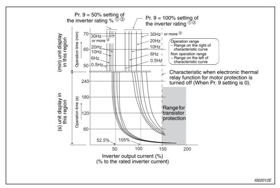
Fig. 6-33: Electronic thermal relay function operation characteristic
