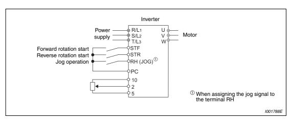
Fig. 6-18: Connection diagram for external jog operation
