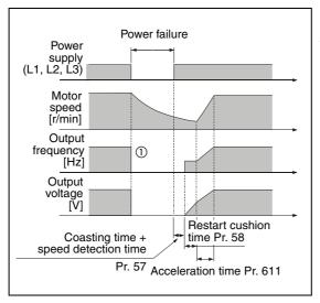
**Fig. 6-69:** Automatic restart with frequency search (Pr. 162 = 0/10)
