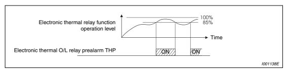
Fig. 6-35: Prealarm signal output
