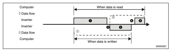
Fig. 6-109: Schematic diagram of data exchange
