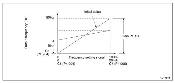
Fig. 6-84: Signal adjustment of terminal 4
