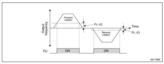
Fig. 6-54: Frequency detection for forward and reverse rotation
