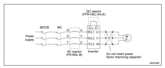
Fig. 3-41: Reduction of power supply harmonics
