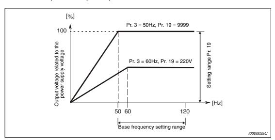
Fig. 6-11: Output voltage related to the output frequency
