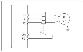
Fig. 6-36: Connection of an external thermal relay
