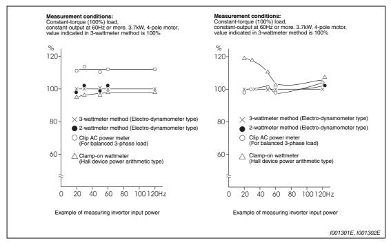
Fig. 7-8: Differences when measuring power with different instruments
