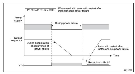
Fig. 6-75: Operation continuation at instantaneous power failure
