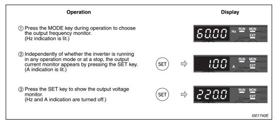
Fig. 4-10: Monitoring of output current and output voltage
