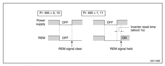
Fig. 6-58: ON/OFF example for source logic
