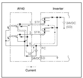
Fig. 3-19: Using an external power supply in connection with the outputs of a PLC (sink logic type)
