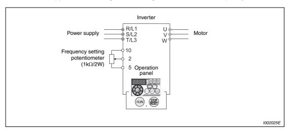
Fig. 5-16: Frequency setting by analog voltage input
