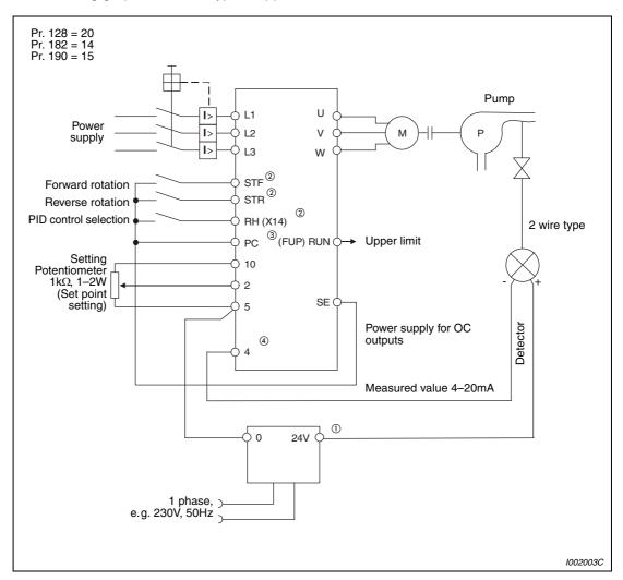
Fig. 6-125: Connection diagram in source logic
