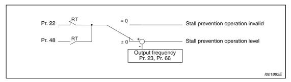
Fig. 6-3: Stall prevention block diagram
