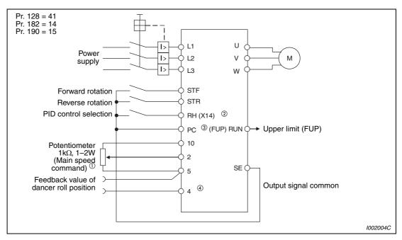
Fig. 6-133: Example in source logic
