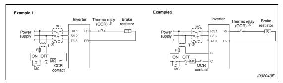
Fig. 3-27: Protection circuits
