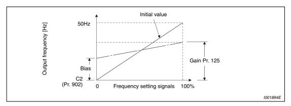
Fig. 6-134: Signal calibration at terminal 2
