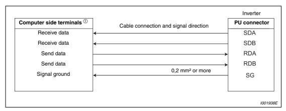
Fig. 6-101: Connection to an inverter
