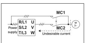
Fig. 4-1: Mechanical interlocks for MC1 and MC2
