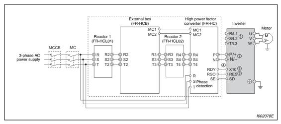
Fig. 3-32: Connection of the high power factor converter FR-HC
