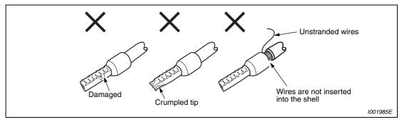
Fig. 3-9: Incorrectly crimped wire end sleeves
