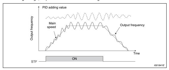
Fig. 6-132: Signal overlay during dancer control
