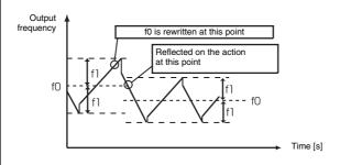
When the output frequency exceeds Pr. 1 Maximum frequency or Pr. 2 Minimum frequency, the output frequency is clamped at maximum/minimum frequency while the set pattern exceeds the maximum/minimum frequency.
