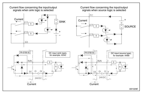
Fig. 3-17: Changing the control logic
