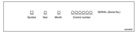
Fig. A-7: Rating plate example
