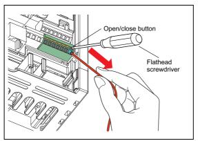
Fig. 3-12: Wire removal
