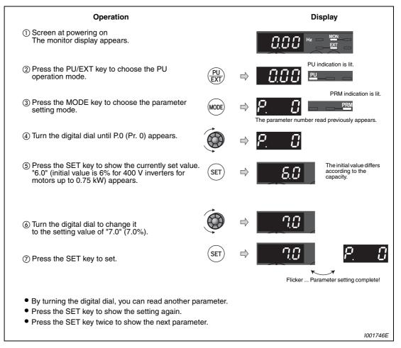
Fig. 5-4: Setting the starting torque
