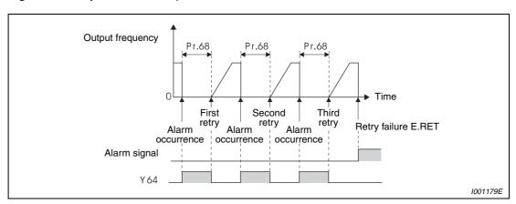
Fig. 6-77: Retry failure example
