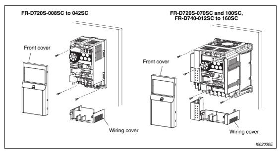
Fig. 2-6: Installation on the panel
