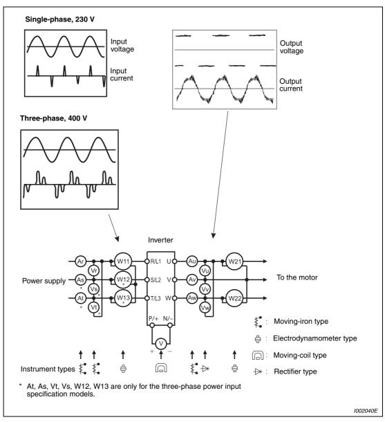
Fig. 8-8: Examples of measuring points and instruments
