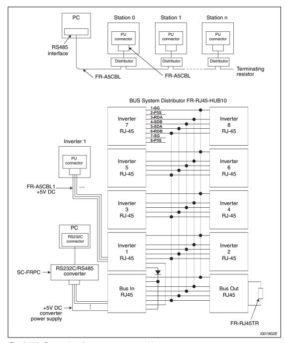
Fig. 6-100: Connection of a computer to several inverters
