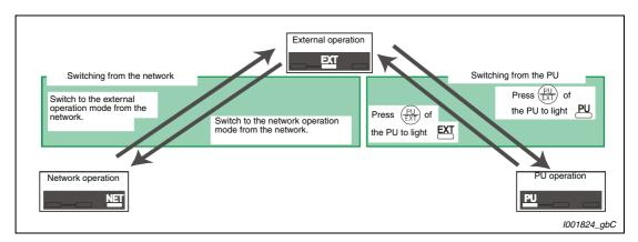
Fig. 6-90: Switching the operation mode when Pr. 340 = 0 or 1
