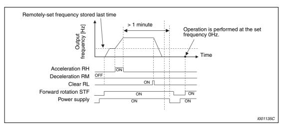
Fig. 6-26: Outputting the current set frequency
