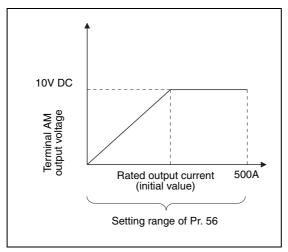
Fig. 6-64: Current monitoring reference
