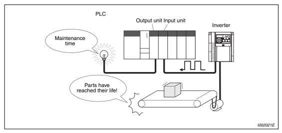
Fig. 6-142: Monitoring the maintenance timer and current average value
