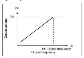
Fig. 6-12: Constant-torque load
