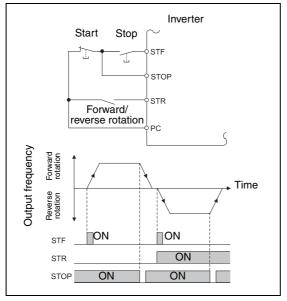
**Fig. 6-50:** 3-wire type connection (Pr. 250 = 8888)
