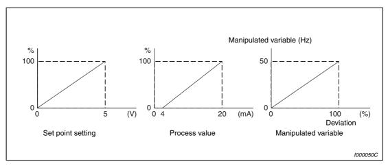
Fig. 6-130: Input calibration
