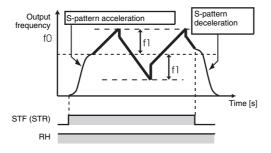
When stall prevention is activated during traverse operation, traverse operation is stopped and normal operation is performed. When stall prevention operation ends, the motor accelerates/decelerates to f0 in normal acceleration/deceleration time (Pr. 7, Pr. 8). After the output frequency reaches f0, traverse operation is again performed.
