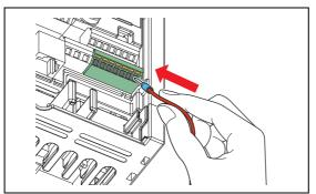
Fig. 3-10: Cable connection
