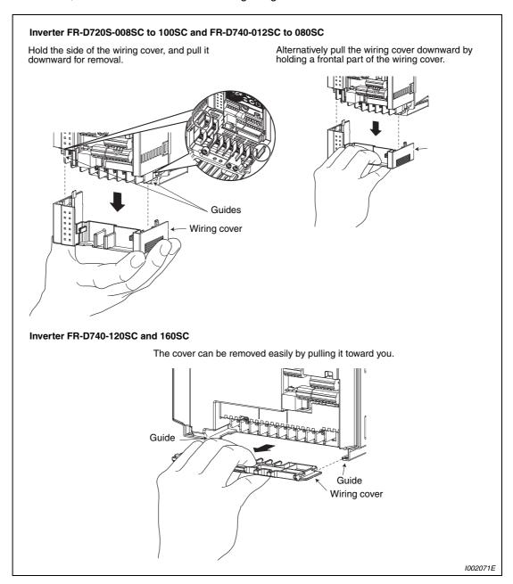
Fig. 2-5: Examples for removing the wiring cover
