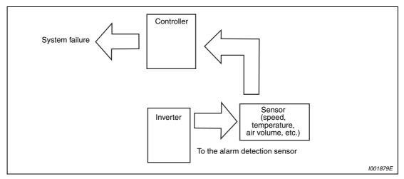
Fig. 4-4: Backup method outside the inverter
