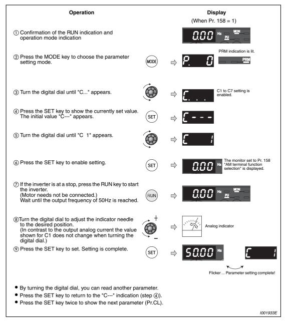
Fig. 6-67: AM terminal calibration
