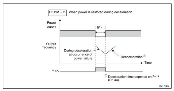
Fig. 6-74: Operation continuation at instantaneous power failure
