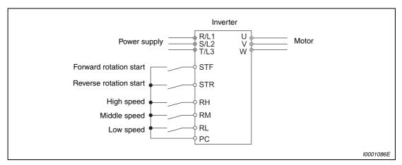
Fig. 5-22: Frequency and start command by switches
