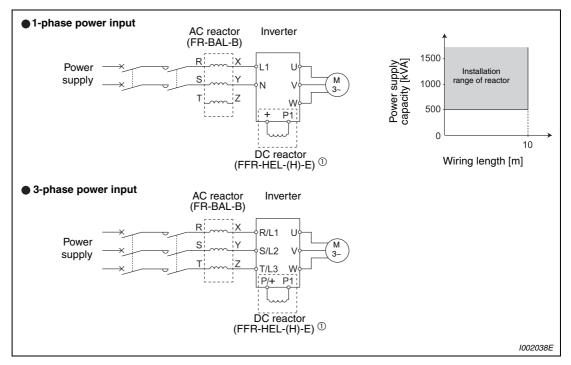
Fig. 3-35: Installation of a reactor
