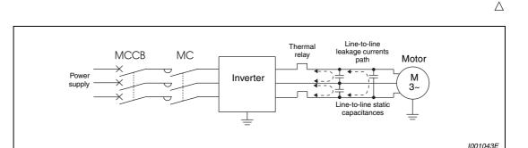
Fig. 3-36: Line-to-line leakage currents
