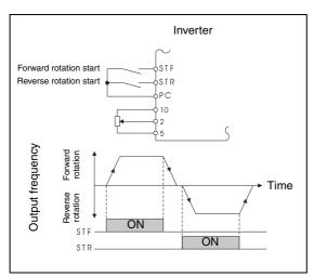
**Fig. 6-47:** 2-wire type connection (Pr. 250 = 9999)
