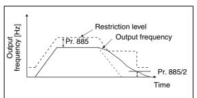
Fig. 6-138: Limit the output frequency
