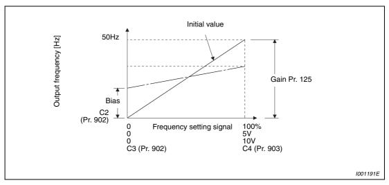
Fig. 6-83: Signal adjustment of terminal 2
