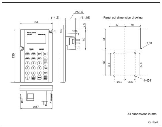
Fig. A-5: Parameter unit FR-PU07
