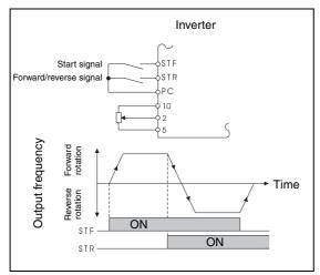
**Fig. 6-48:** 2-wire type connection (Pr. 250 = 8888)
