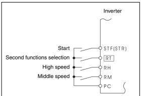
Fig. 6-45: Second functions connection diagram
