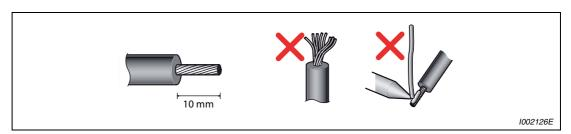
Fig. 3-7: Preparation of the cable
