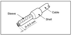
Fig. 3-8: Fixing of wire end sleeves
