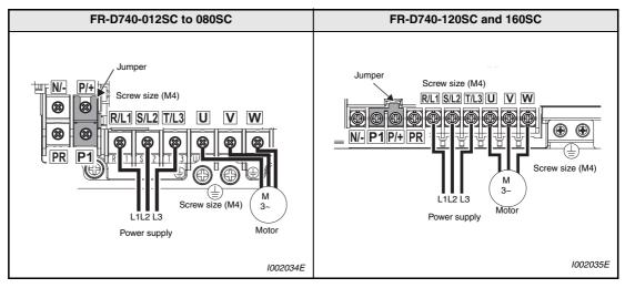
Tab. 3-4: Terminal layout and wiring
