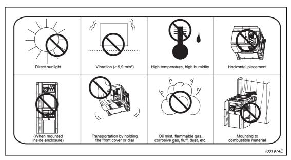
Fig. 2-8: Conditions, that could cause an operation fault or failure
