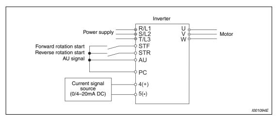
Fig. 5-28: Frequency setting by analog current input
