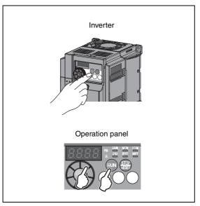
Fig. 6-93: PU operation mode
