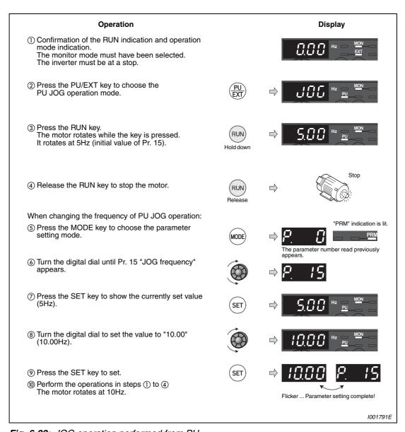
Fig. 6-22: JOG operation performed from PU
