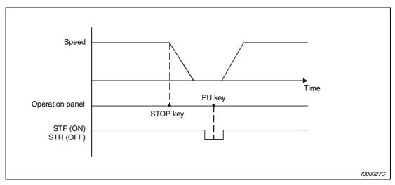
Fig. 6-88: Stop during external operation
