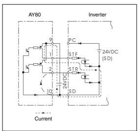
Fig. 3-20: Using an external power supply in connection with the outputs of a PLC (source logic type)
