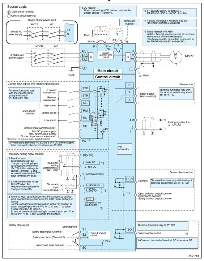
Fig. 3-3: Terminal connection diagram of the inverter
