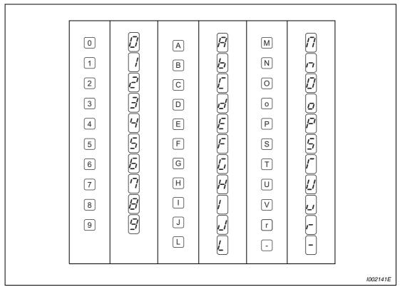
Fig. 7-4: Correspondences between digital and actual characters (operation panel)
