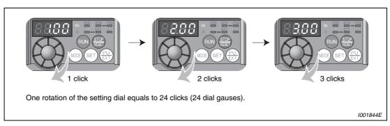
Fig. 6-146: Magnitude when parameter 295 is set to "1.00"
