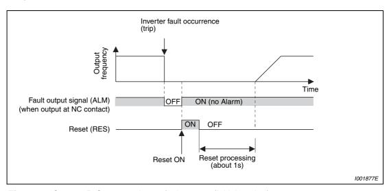
Fig. 4-2: Contact B-C opens when a fault occurs (initial setting)
