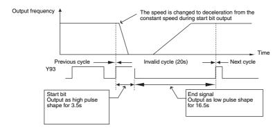
When the output current value (inverter output current monitor) is 0A on completion of the 1 cycle signal output, the signal is not output until the speed becomes constant next time.
