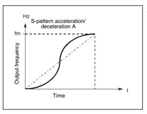
Fig. 6-31: Characteristic for parameter 29 = 1
