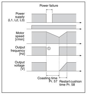
Fig. 6-68: Automatic restart without frequency search (Pr. 162 = 1/11)
