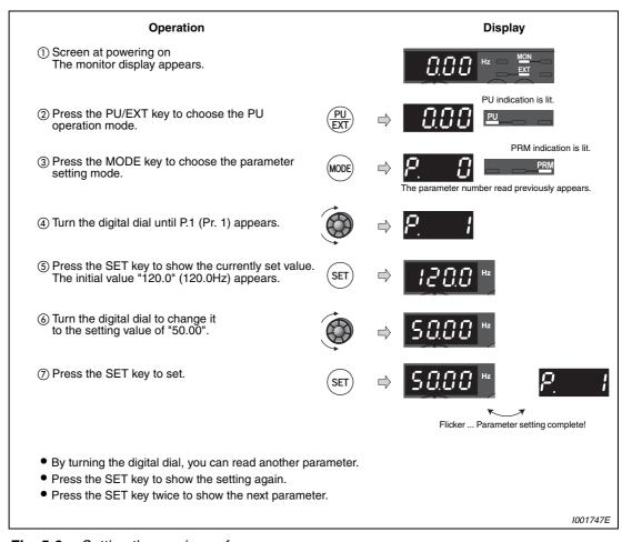
Fig. 5-6: Setting the maximum frequency
