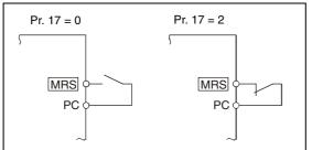
Fig. 6-44: Connection of the MRS terminal in source logic
