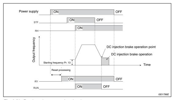
Fig. 6-51: Ready and motor running signals
