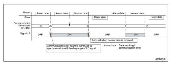
Fig. 6-118: Output of the LF signal
