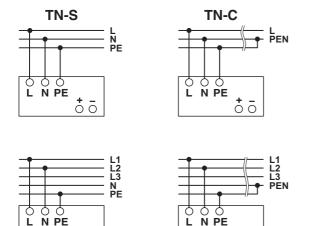
The 100 ... 240 V AC connection is established using the L, N and PE screw connections.
