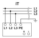
The connection for  $3x\ 400\ V\ AC\ ...\ 500\ V\ AC$  is established using the L1, L2, L3 and PE screw connections. The device can be connected to a 3-phase system with nominal voltages of  $3x\ 400\ V\ AC\ ...\ 500\ V\ AC$ . In the event of a phase failure, unrestricted operation is possible with nominal capacity.
