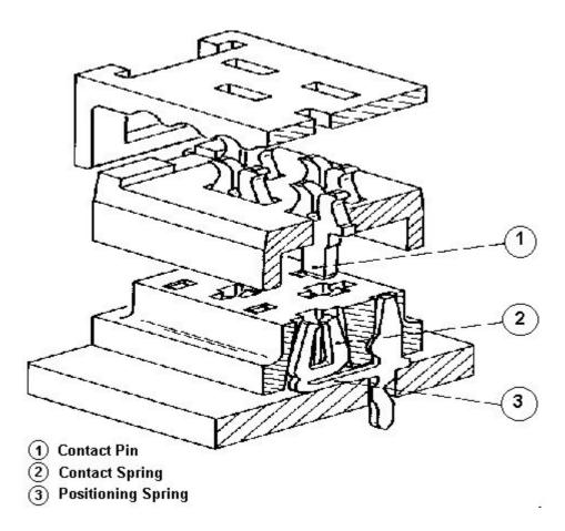
The Micro-MaTch contact spring system is absolutely fretting corrosion proof by its design.
