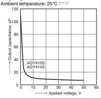
12-(2). Output capacitance vs. applied voltage characteristics
