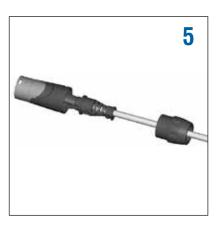
Push clamp-boot & cable together into the shell
