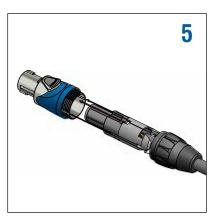
Orientate the insert and cable clamp as shown then push all together into the shell.
