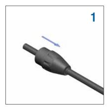
Slide the nut (Backshell) onto the cable
