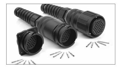
Amphenol's MP-41 series of multipin connectors utilise the same design principals of the rugged Mil-C-5015 military connectors. They can withstand high shock and vibration environments and are ideal for tough on-road applications. Featuring a quick mating bayonet coupling with an audible full mating feature ensures a positive connection every time. Available from 13 to 150 pins with contacts supplied with each connector as standard.
