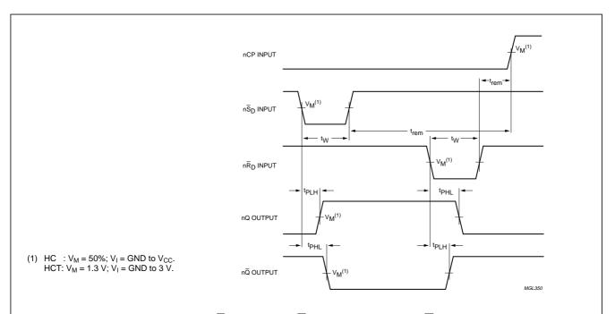
Fig.7 Waveforms showing the set  $(n\overline{S}_D)$  and reset  $(n\overline{R}_D)$  input to output  $(nQ, n\overline{Q})$  propagation delays, the set and reset pulse widths and the  $n\overline{R}_D$ ,  $n\overline{S}_D$  to nCP removal time.
