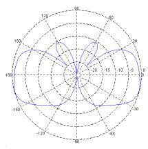
Elevation (E-field) radiation pattern
