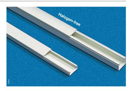
TMK-T20 is a halogen-free mini-trunking for quick and simple concealed installation of cables and wires for signals and power, data, telecoms and alarms. It is fixed directly to the surface with penetrating fixings in pre-punched holes. Alternatively it can be secured with adhesive (only permitted with low-current wiring).
