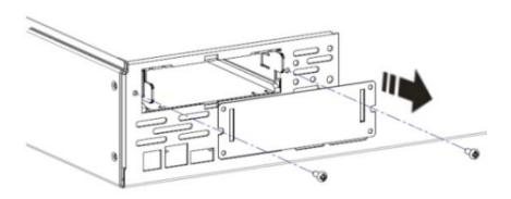
3. Orient the Card to fit in the Card slot as shown. Slide the Card all the way into the slot until the end plate is flush with the back panel of the host device.
