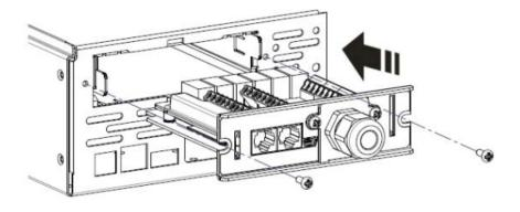
Trying to install the Card upside down may damage it. Observe the correct orientation of the Card. The sides of the printed circuit board align with the guides in the sides of the Card slot. The slot may be oriented horizontally or vertically in the host device, which must be off.
