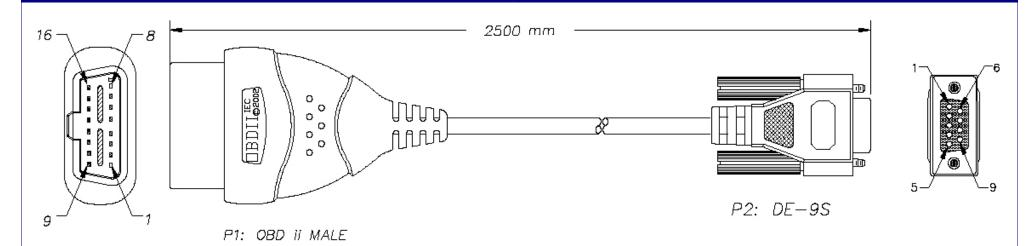
Connector P1: Molded OBD II Male Connector for Type B (24 Volt) and Type A (12 Volt)
