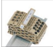
The group label holder **ZSchT 4** can be swivelled and is attached to the support bracket **ZES 35**. It is parallel to the mounting rail. The insertion label **ESO** and the protective strip **STR** complete the holder.
