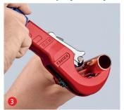
Tighten and cut with a swift twist and then readjust using the ergonomic blue feeding barrel
