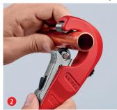
Push the cutting wheel against the pipe with the QuickLock single hand quick adjustment: fastest adjustment to different pipe diameters
