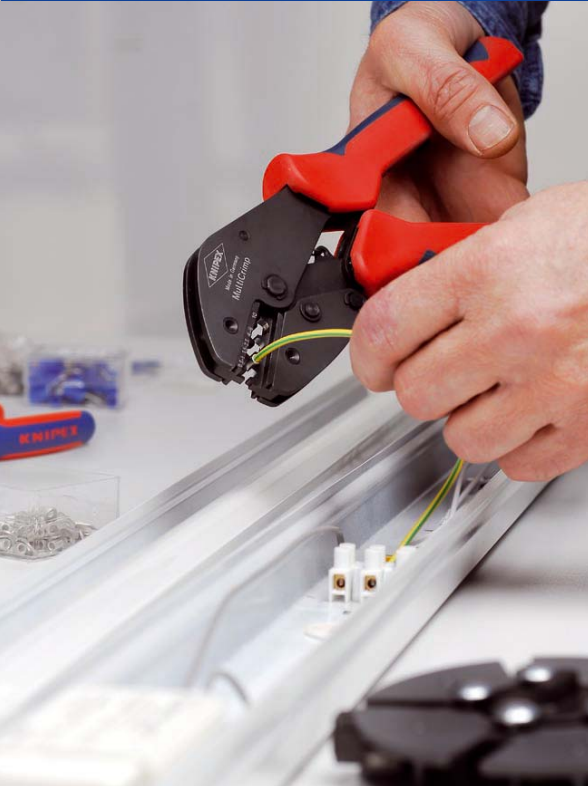
Secure attachment of the dies in the pliers by reliable locking system
