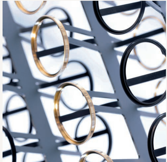
The picture shows precision-engineered brass mounts in a jig, prepared for surface treatment. To avoid reflections, the mounts are chrome-plated in matte black.
