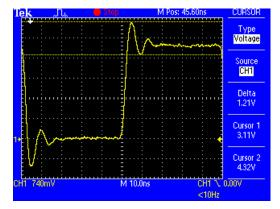
The higher the bandwidth, the more accurate the reproduction of your signal, as illustrated with a signal captured by the TDS2000 Series at 60 MHz and 200 MHz bandwidth levels.
