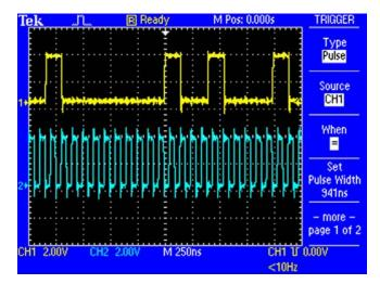
Setting the pulse width to = 941 ns enables you to capture signals with widths equal to 941 ns wide on channel 1 using the TDS2000 Series.
