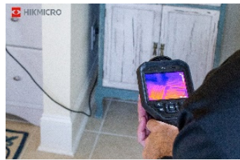
Check Underfloor Heating
