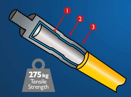
1 Glued 2 Indented 3 Crimped
