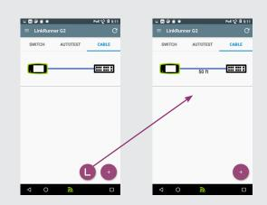
Like the LinkRunner AT, the LinkRunner G2 can generate a digital tone compatible with the Intellitone<sup>™</sup> probe to trace the cable around the patch panel/cross-connect while the cable is connected to the Switch. If the connected switch supports CDP/LLDP, the LinkRunner G2 can also show the switch name and port connected, making cable tracing at the IDF even more straight forward.
