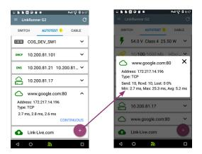
Conduct a "TCP Connect" test to an unlimited number of IP devices. Use the "CONTINUOUS" function to perform the test continuously to assess connectivity and response time consistency of a target.
