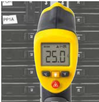
IR thermometer, temperature measurement in one spot
