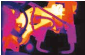
Hot spot in welding robot
