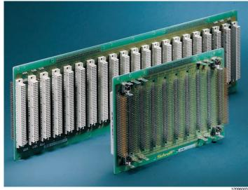
Universal backplanes without through-connected signal lines, 10 and 21 slot
