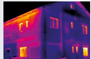
Detect energy losses from buildings: immediately identify and record thermal bridges in building fronts or shells.
