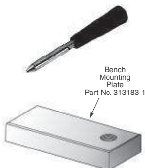
Shielding Enclosure Expansion Tools Part No. 58241-1 (.450 [11.43])† 58241-2 (.572 [14.53])† 58241-4 (.330 [8.38])† †Maximum Cable Diameter (Instruction Sheet—408-9507)
