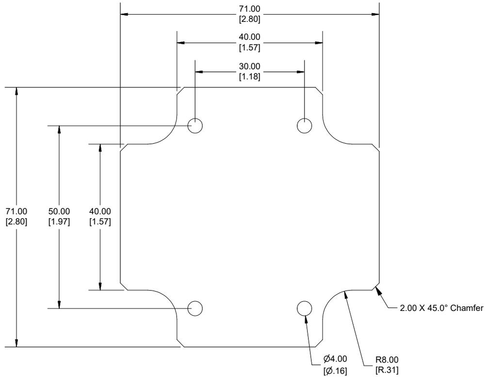
Enclosures can be Factory Modified (Milling, Drilling, Printing etc.)
