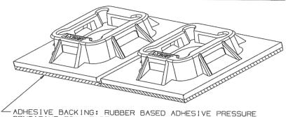
ADHESIVE BACKING: RUBBER BASED ADHESIVE PRESSURE SENSITIVE FOAM TAPE 0.04 [1.0] THICK WITH A PROTECTIVE LINER. MOUNT IS DESIGNED TO SUPPORT 0.50 lbs (227g) MAX. WEIGHT ON A CLEAN DRY SMOOTH SURFACE.
