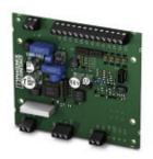
The EV-CC-AC1-M3-CBC-SER-PCB charging controller as PCB is used for charging electric vehicles at 3phase AC networks according to IEC 61851-1, Mode 3. Optimized for charging stations with permanently mounted Vehicle Connector. All charging functions and comprehensive configuration settings are already integrated.
