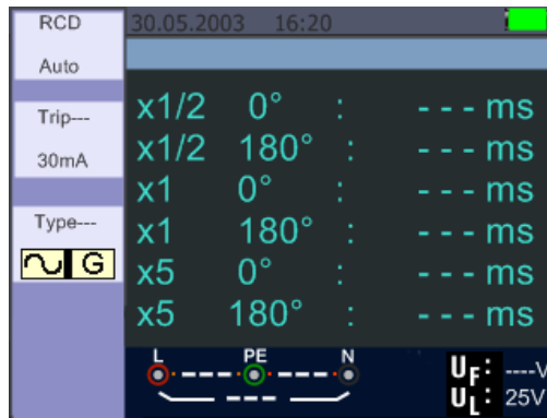
RCD – Standby screen
