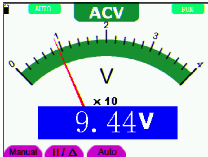
figure 23: AC Voltage Measurement
