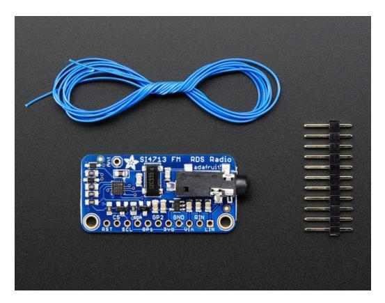
This transmitter even has RDS/RBDS support - that's text/data transmissions that many modern FM receivers support. (It's how some car radios can display the FM station and current song playing). You can transmit just about any text you want, set the station identifier as well as the 'freeform' buffer.
