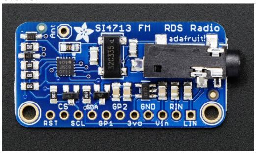
Yaaar! Become your very own pirate radio station with this FM radio transmitter. This breakout board, based on the best-of-class Si4713, is an all-in-one stereo audio FM transmitter that can also transmit RDS/RBDS data!
