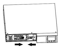
Re-connect the battery wires.
