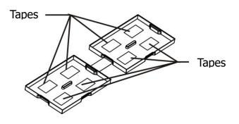
Step 3: Put assembled battery packs on one side of plastic shells.
