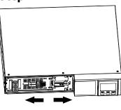
Disconnect battery wires.
