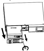
Pull out the battery box by removing two screws on the front panel.
