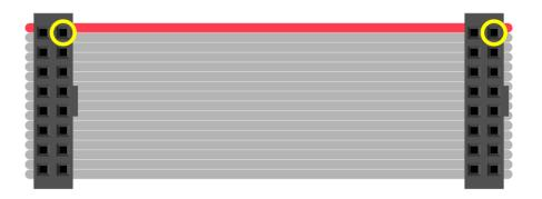
Plugged into a socket on the LED matrix, one header now faces *away* from you. If you double the cable back on itself (not a twist, but a fold)...to access a specific pin on the socket, the left and right columns are now mirrored (rows are in the same order — the red stripe provides a point of reference). You're looking "up" into the plug rather than "down" into the socket.
