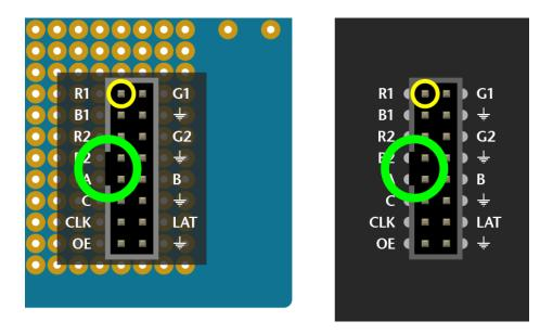
Wires are then soldered from the header to specific Arduino pins on the proto shield. Try to keep wire lengths reasonably short to avoid signal interference.
