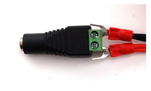
You may receive power cables with different endings, e.g. round instead of spade ends, or maybe with another Molex connector. Just strip the cables and wire directly to the power plug
