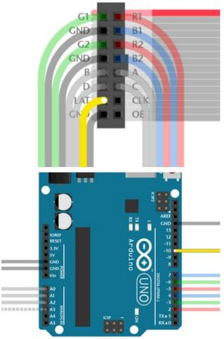
The LAT signal connects to Arduino pin 10.
