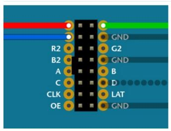
Pins **R1**, **G1** and **B1** (labeled R0, B0 and G0 on some matrices) deliver data to the **top half** of the display.
