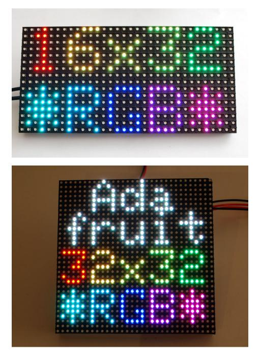
These panels require 12 or 13 digital pins (6 bit data, 6 or 7 bit control) and a good 5V power supply, at least a couple amps per panel. We suggest our 2A (or larger) regulated 5V adapters and either a terminal block DC jack, or solder a jack from our DC extension cord. Please read the rest of our tutorial for more details!
