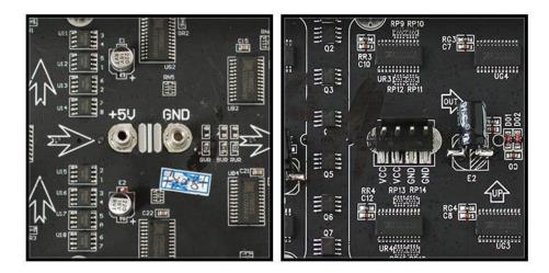
On the left is a screw post power connector (with adjacent pads for soldering wires directly). On the right, a Molex-style header. Some panels will have *two* headers...the power cable included with these panels has connectors for both headers.
