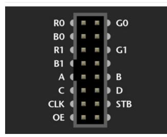
"Variant B" for 32x32 and 64x32 panels. The wiring is *identical* to Variant A above, *only the labels* are different.
