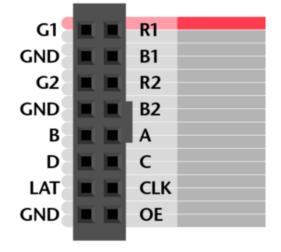
Either end of the ribbon cable can be plugged into the matrix INPUT socket. Notice below, the "key" faces the same way regardless.
