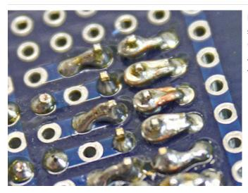
Depending on the make and model of proto shield, some pins are designed to connect in short rows. Others don't. For the latter, strip a little extra insulation and bend the wire to wrap around the leg of the socket from behind, then solder.
