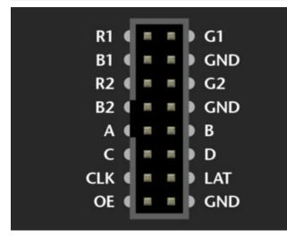
Here's the layout for **32x32** and **64x32** panels. We'll call this "**Variant A**." Some panels use different labels, but the functions are identical.
