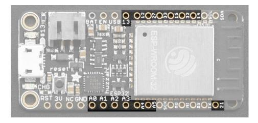
There are tons of GPIO and analog inputs available to you for connecting LEDs, buttons, switches, sensors, etc. Here's the remaining pins available.
