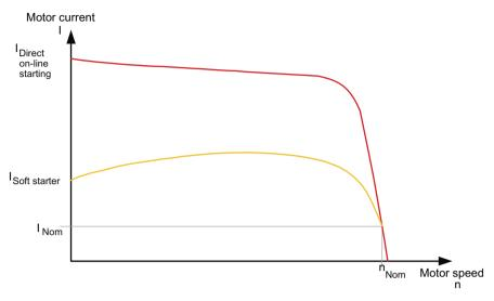
Figure 3-3 Reduced current characteristic of a three-phase induction motor during starting with a SIRIUS 3RW30 or 3RW40 soft starter
