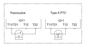
Figure 15-1 Optional thermistor motor protection evaluation
