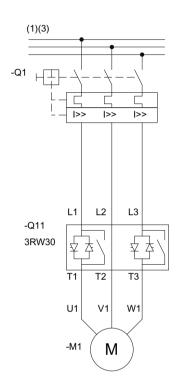
Figure 15-8 Wiring of the 3RW30 control and main circuits
