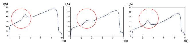
Figure 3-6 Current characteristic and occurrence of DC components in the three phases without "polarity balancing"
