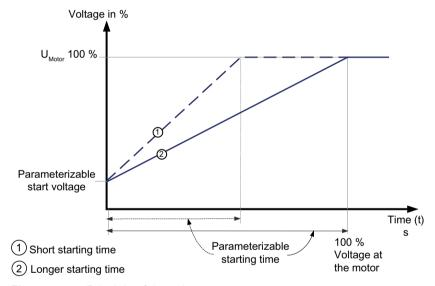
Figure 5-1 Principle of the voltage ramp
