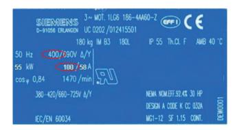
The rated operational current of the motor must be set with the  $I_e$  potentiometer according to the mains voltage and the motor connection (wye-delta). The electronic motor overload protection also refers to this set value if it is active. For the permissible settings referred to the required motor overload trip class, refer to chapter Motor current settings (Page 113).
