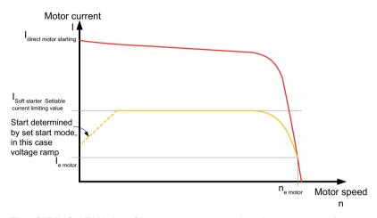
The SIRIUS 3RW40 soft starter measures the phase current (motor current) continuously with the help of integrated current transformers.
