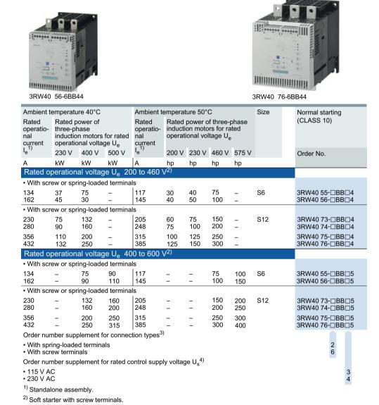
3) Main circuit connection: busbar connection.
