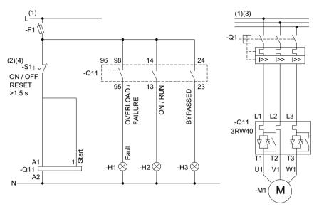
Figure 15-9 Wiring of the 3RW40 2 to 3RW40 4 control circuit and the 3RW40 2 to 3RW40 7 main circuit
