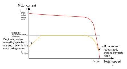
Figure 5-4 Current limiting with soft starter
