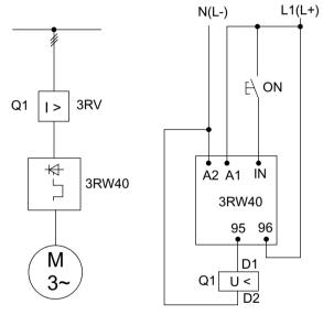
Figure 5-6 3RW40 wiring fault with 3RV
