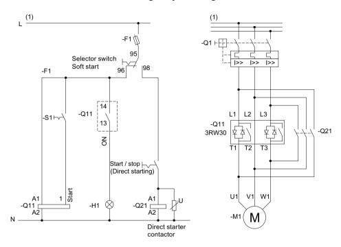
Figure 15-29 Wiring of the 3RW30 control and main circuits
