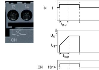
State diagram of the ON output contact
