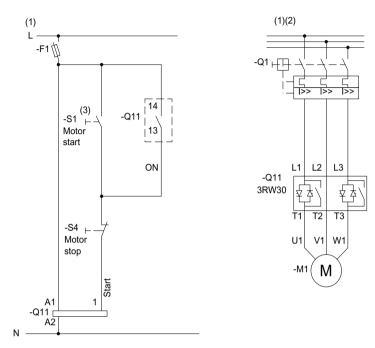
Figure 15-2 Wiring of the 3RW30 control and main circuits
