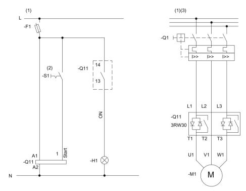
Figure 15-5 Wiring of the control and main circuits
