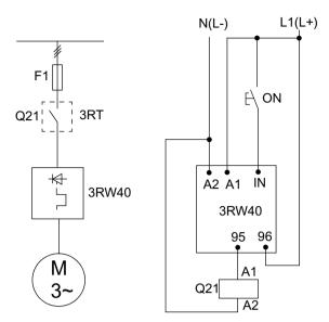
Figure 5-5 3RW40 wiring fault
