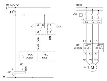
Figure 15-11 Wiring of the 3RW30 control and main circuits
