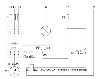
12.10 RESET MODE and functions of the RESET / TEST button
