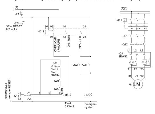
Figure 15-28 Wiring of the 3RW40 5 to 3RW40 7 control circuit and the 3RW40 2 to 3RW40 7 main circuit
