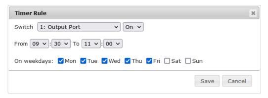
You set here which port should be switched for which time period, and on which days of the week the rule is active. In this example the period 9:00 to 17:00 is changed to 9:30 to 11:00 compared to the default input mask. Also, this rule should not be applied on Saturday and Sunday. The rule we have now says that every day, except Saturday and Sunday, port 1 will be switched on at 9:30 and switched off after 1.5 hours. Clicking on "Save" saves this rule.
