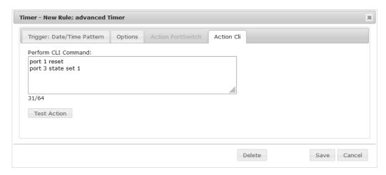
Instead of switching a port, one or more console commands can be executed. These commands are entered in the "Action CLI" register. The "Action Cli" tab can only be selected if the option "Perform CLI Cmd" is activated in "Options".
