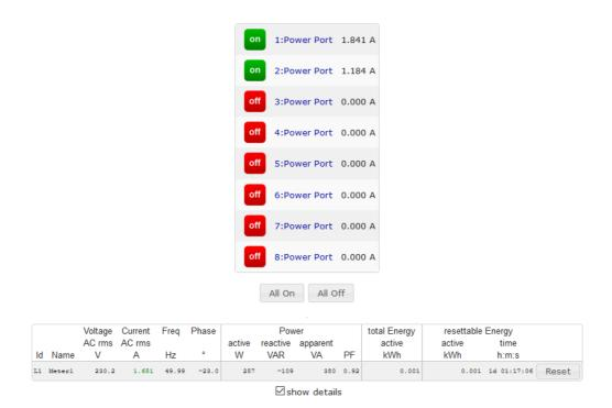
The web page provides an overview of the switching state, energy measurement values, as well as the external sensors, provided that they are connected. When a single port is clicked a panel with buttons to control a single port appear:
