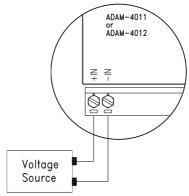
Figure 8-1 Applying Calibration Voltage
