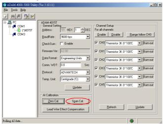
7. Apply 10K ohms resistor with 0.01% accuracy to CH0 and then Click on "Save"
