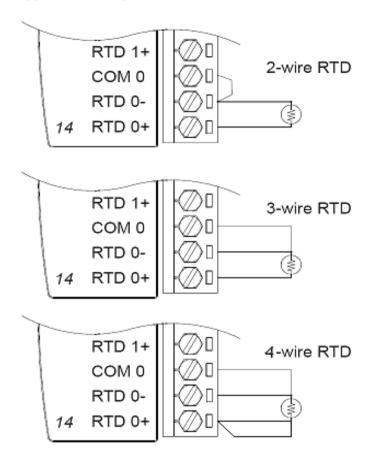
Figure 3-18 ADAM-4015 RTD Input Module Wiring Diagram
