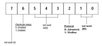
Figure 7-1 Data format for FF (8-bit parameter)
