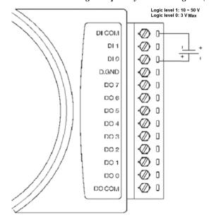
Figure 3-55a ADAM-4055 Digital Input Wet Contact Wiring Diagram
