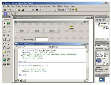
**Step 10.** Run the Project  $\rightarrow$  Click OPEN to open COM1  $\rightarrow$  Click SEND to send the Get Temperature Reading Command. Now, you will find the reading the same as the displayed format shown below.
