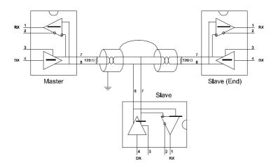
Figure E-5 Termination resistor locations
