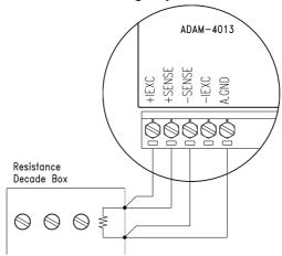
Figure 8-5 Applying calibration resistance
