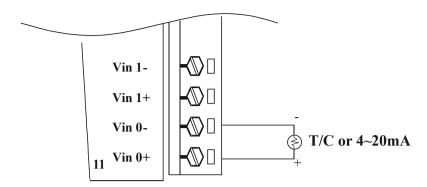
Figure 3-33 ADAM-4018+ Thermocouple Input Wiring Diagram
