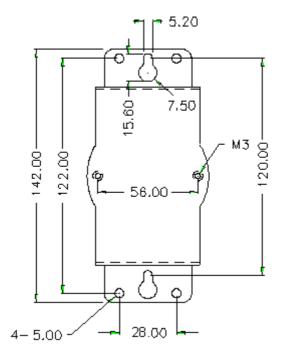
Figure C-4 Panel Mounting Bracket Dimensions
