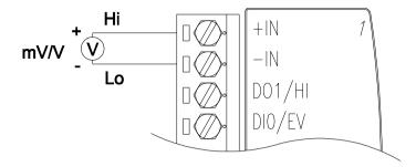
Figure 3-10 ADAM-4012 Millivolt and Volt Input Wiring Diagram
