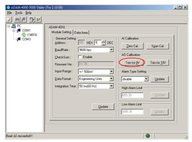
Figure 8-8 Zero Calibration
