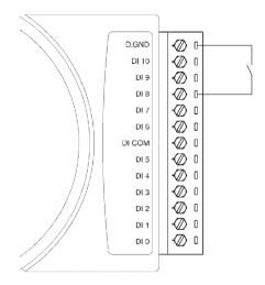
Figure 3-45 ADAM-4051 Dry Contact Wiring Diagram
