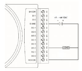
Figure 3-53 ADAM-4055 Digital Output Wiring Diagram
