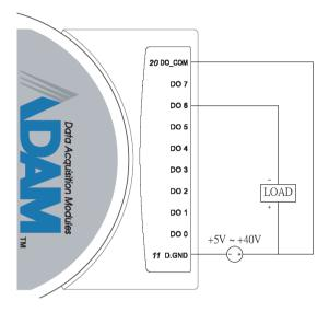
Figure 3-58 ADAM-4056S Digital Output Wiring Diagram
