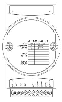
Figure 3-36 ADAM -4021 Analog Output Module
