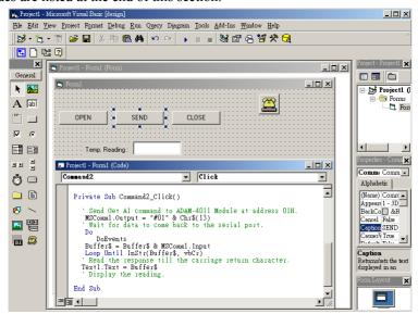
**Step 9.** Click CLOSE Button and type in the following codes. The source codes are listed at the end of this section.
