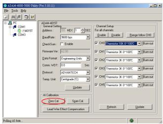
5. Apply 800.0 ohms resistor with 0.01% accuracy to CH0 and then Click on "Save"
