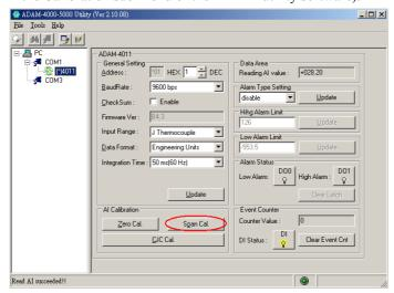
Figure 8-3 Span Calibration
