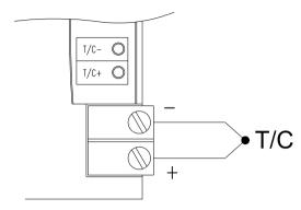
Figure 3-3 ADAM-4011/4011D Thermocouple Input Wiring Diagram
