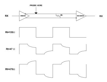
Figure E-4 Signal Distortion
