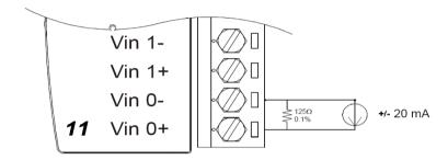
Figure 3-30 Current Input Wiring Diagram of ADAM-4017
