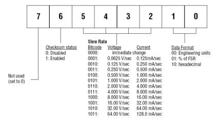
Figure 6-1 Data format for FF (8-bit parameter)
