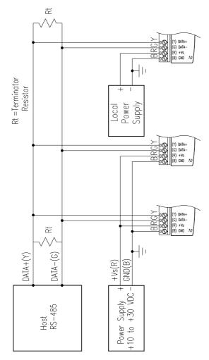
Figure 2-5 Multi-module Connection
