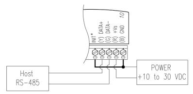
Figure 2-3 Grounding the INIT\* Terminal
