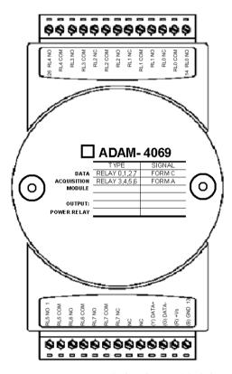
Figure 3-67 ADAM-4069 Relay Output Module
