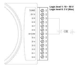
Figure 3-46 ADAM-4051 Wet Contact Wiring Diagram
