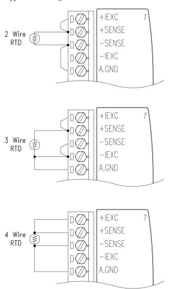
Figure 3-16 ADAM-4013 RTD Inputs Wiring Diagram
