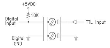
Figure 3-41 ADAM-4050 TTL Input Wiring Diagram
