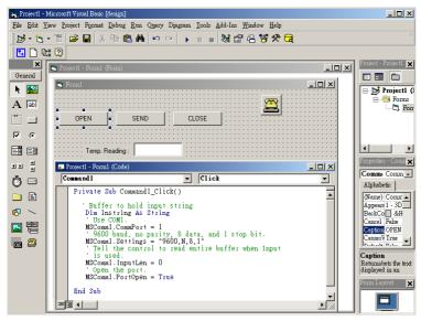
**Step 8.** Click SEND Button and type in the following codes. The source codes are listed at the end of this section.
