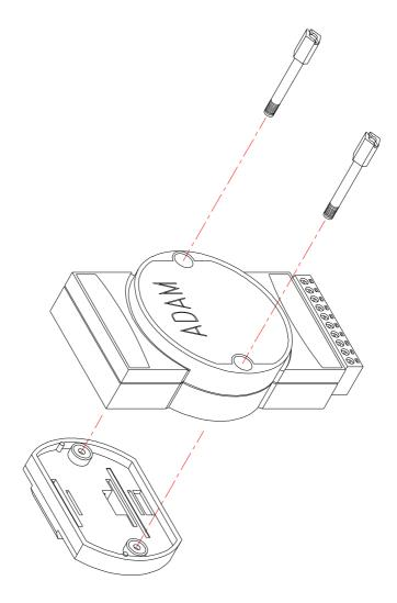
Figure C-2 DIN-Rail Adapter
