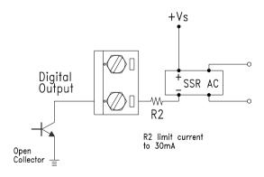
Figure 3-12 ADAM-4012 Digital Output Wiring Diagram
