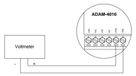
Figure 8-7 Setup for Voltage Output Calibration
