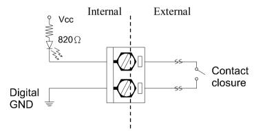
Figure 3-51 ADAM-4053 Contact Closure Input Wiring Diagram
