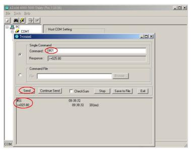
Figure D-4 Terminal Function
