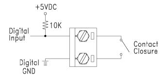
Figure 3-8 ADAM-4011/4011D Digital Input Wiring Diagram
