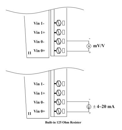
Figure 3-32 ADAM-4017+ Voltage and Current Input Wiring Diagram
