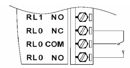
Figure 3-68 ADAM-4069 Form C Relay Output
