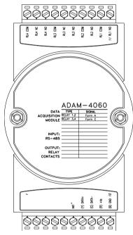
Figure 3-61 ADAM-4060 4-channel Relay Output Module
