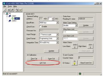
Figure 8-4 Cold Junction Calibration
