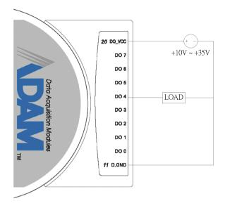
Figure 3-60 ADAM-4056SO Digital Output Wiring Diagram
