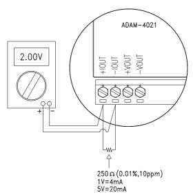
Figure 8-6 Setup for Analog Output Calibration
