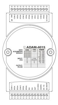
Figure 3-17 ADAM-4015 6-channel RTD Input Module
