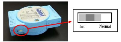
Figure 2-4 Set INIT switch to "Init"
