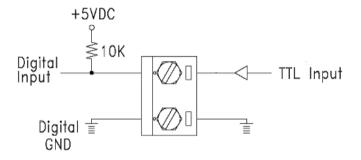
Figure 3-7 ADAM-4011/4011D Digital Input Wiring Diagram
