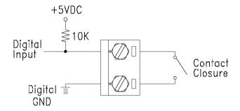
Figure 3-14 ADAM-4012 Digital Input Wiring Diagram
