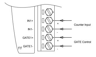
Figure 3-73 ADAM-4080/4080D Photo-isolated Input
