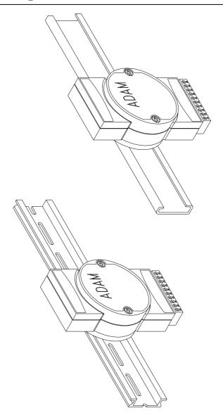
Figure C-3 DIN-Rail Mounting
