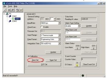
Figure 8-2 Zero Calibration
