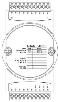
Figure 3-40 ADAM-4050 Digital I/O Module
