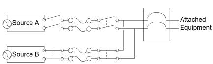
**NOTE:** The entire switching process (described in step 2) takes a maximum of 10 milliseconds (ms) at high sensitivity, and 12 ms at low sensitivity.
