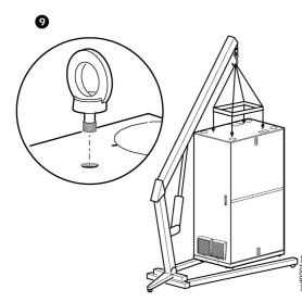
**NOTE:** Remove the eye bolts and replace the hole plugs when the lifting task is complete.
