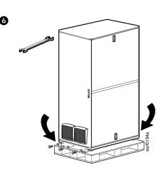
7. Remove the two (2) M8 x 14 mm bolts securing each bracket to the pallet at the front and rear.
