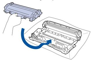
7. Install the toner cartridge and drum unit assembly back into the machine.
