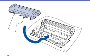
Make sure you put the toner cartridge in correctly or it may separate from the drum unit.
