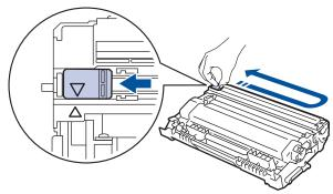
Be sure to return the tab to the Home position (▲). The arrow on the tab must be aligned with the arrow on the drum unit. If it is not, printed pages may have a vertical stripe.
