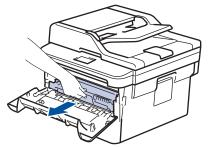
4. Push down the green lock lever and take the toner cartridge out of the drum unit.
