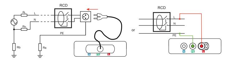
The instrument first of all checks that the voltage between the L and PE terminals is correct. If it is, the symbol lights steadily. If not, the symbol blinks and it is not possible to make a test. If  $U_{LPE} < 90$  V, the instrument displays  $U_{LPE}$  and  $U_{NPE in}$  alternation.
