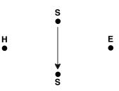
Avoid routing the connecting cables of the earth rods near or parallel to other cables (transmission or power supply), metal pipes, rails, or fences, this in order to avoid the risk of cross-talk with the measurement current.
