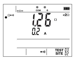
For as long as the measurement varies between some value and **OL**, the instrument remains on even if not in permanent mode **P**.
