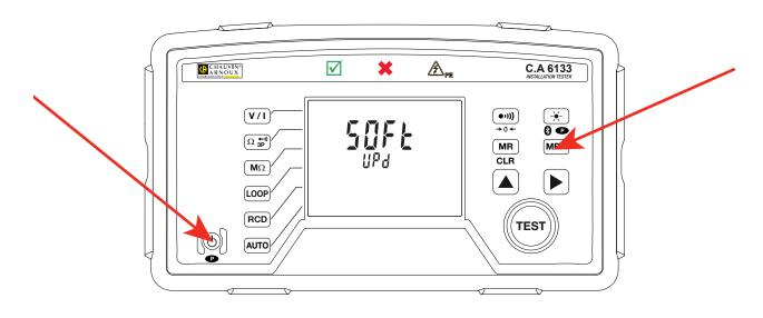
Updating the embedded software erases the recorded data and the configuration of the instrument. As a precaution save the data to a PC before updating the embedded software.
