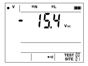
In the case of a live measurement (LOOP or RCD), the instrument shows where the phase should be on the outlet using the  $\ddagger$  symbol. If the phase is on the wrong side, the  $\ddagger$  or  $\ddagger$  symbol blinks to indicate that the tripod cable must be reversed.
