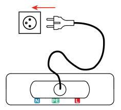
The measurement is displayed. The instrument indicates that it is making the measurement between the L and N terminals. It is therefore possible to make the measurement with two leads.
