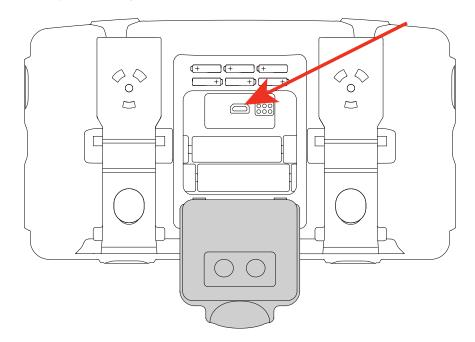
Simultaneously press the <sup>(1)</sup> button and the MEM key (for the C.A 6133) or the <sup>(2)</sup> key (for the C.A 6131). The instrument displays SOFt UPd.
