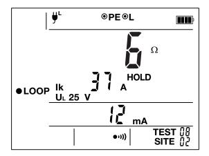
The measurement starts automatically. The result is displayed: the loop impedance and the short-circuit current (lk). Press the **TEST** key to return to voltage measurement.
