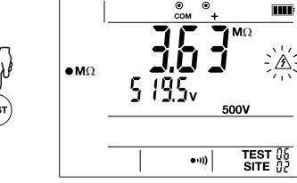
When you release the **TEST** button, the instrument displays **dIS** (discharge) to indicate that it is discharging the object tested. If the object is not capacitive, discharging is very rapid. When the voltage falls below 25V, the **dIS** and A symbols disappear from the display unit.
