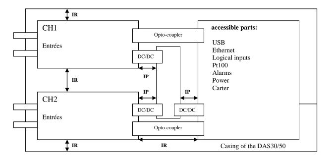
IP: Main or additional insulation IR: Reinforced insulation
