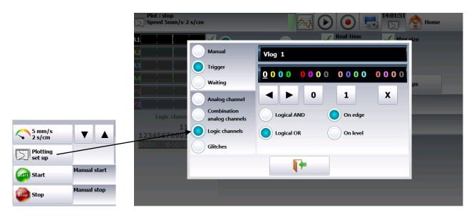
The 16 logic channels can be used in the trigger word:
