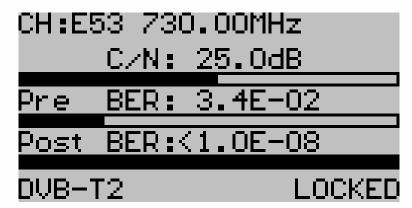
Hopefully, but not always, the digital readout; BER (bit error rate) and C/N (Carrier/Noise) will correspond well with the analog setting of the antenna. Quite often the antenna needs to be re-directed a little bit in order to maximize the digital-values (which are of more importance then the analog readout).
