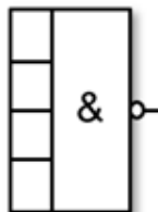
Figure 10-27 Logic gate with NAND operator
