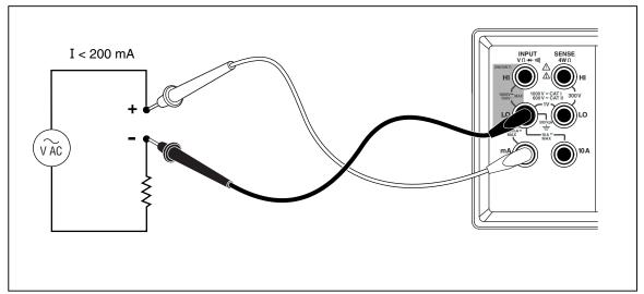
Figure 3-8. Current Measurement <200 mA
