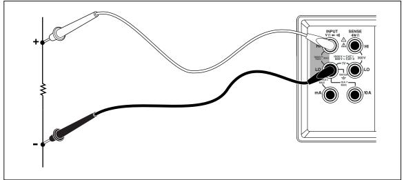
Figure 3-5. 2-Wire Resistance Measurement
