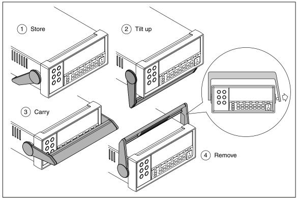
Figure 2-4. Bail Adjustment and Removal
