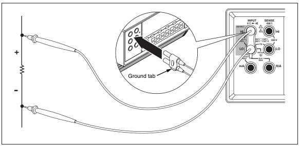
Figure 3-7. Input Connections for 4-Wire Ohms Using 2x4 Wire Leads
