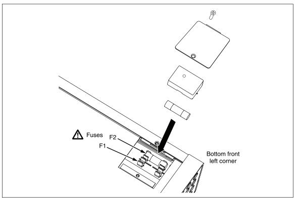
Figure 2-2. Replacing the Current-Input Fuses
