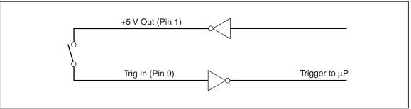
Figure 3-12. External Trigger Circuit
