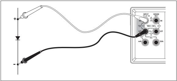
Figure 3-11. Diode Test
