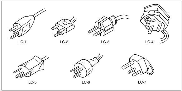
Figure 2-3. Line-Power Cord Types Available from Fluke
