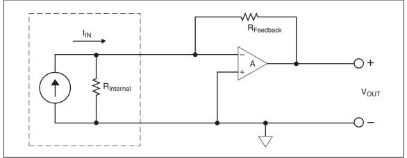
Figure A-4. Zero Burden Voltage Low-Level Current Measurement
