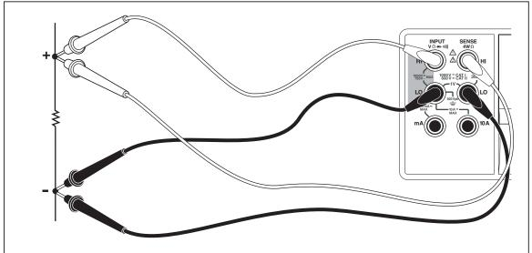
Figure 3-6. 4-Wire Resistance Measurement
