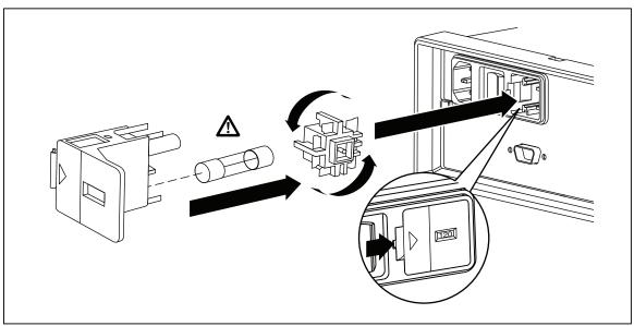
Figure 2-1. Replacing the Line Power Fuse
