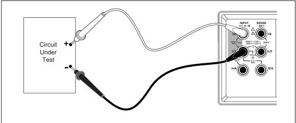
Figure 3-4. Voltage and Frequency Measurement
