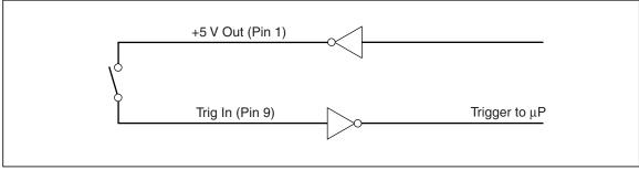
Figure 4-1. External Trigger Using Pin 9 of RS-232 Interface
