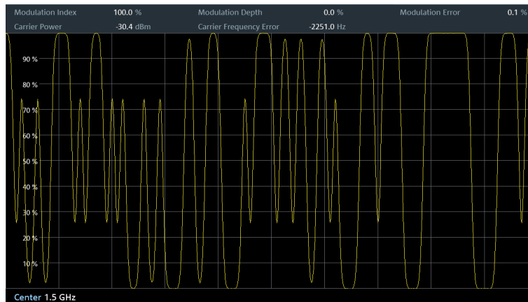
Figure 18-4: Modulation depth of a 2ASK signal
